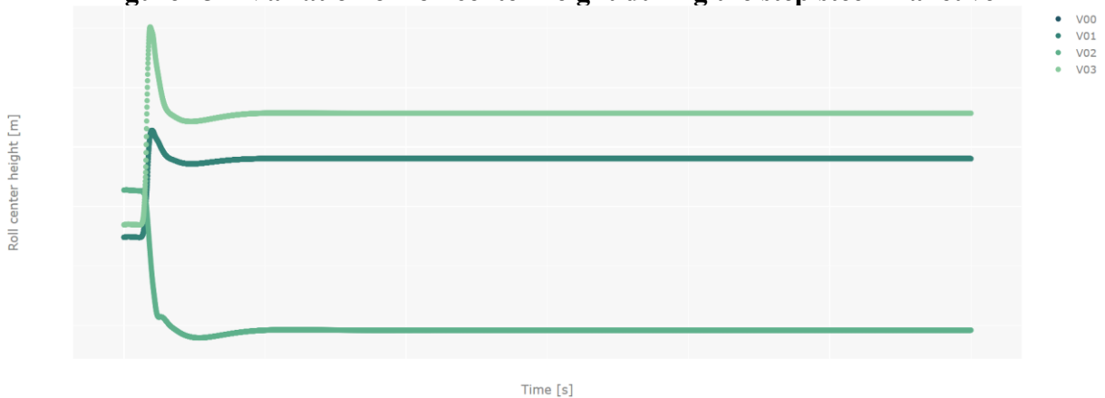
Figure 43 – Variation of roll center height during the step steer maneuver
