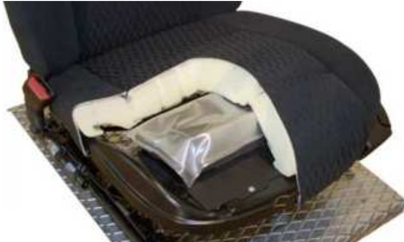
Figura 2.12 – Sistema anti-sliding bag (AUTOLIV Anti-sliding bag, 2002)
