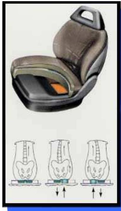
Figura 2.15 – Sistema Comfort Renews (JOHNSON CONTROLS Renews, 2009).
