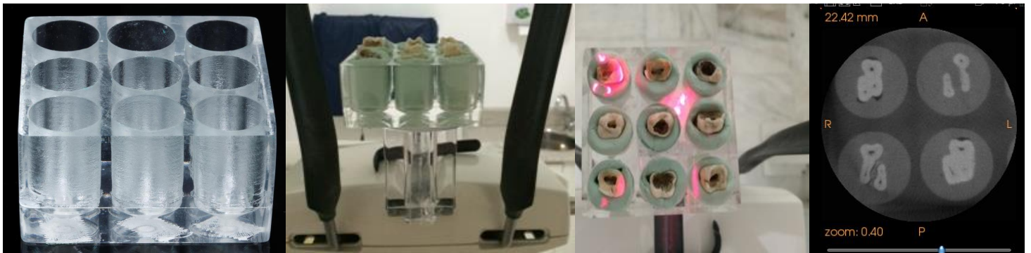
Figure 1. Examination of standardization CBCT: A- Acrylic plate with nine holes B- Acrylic plate on the table of the tomograph C- Tomography and examination D- Axial image of CBCT.
