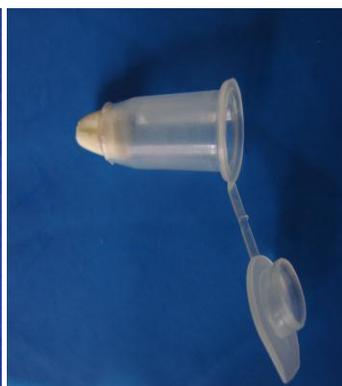
**Figura 15** - Impermeabilização com Cianoacrilato
