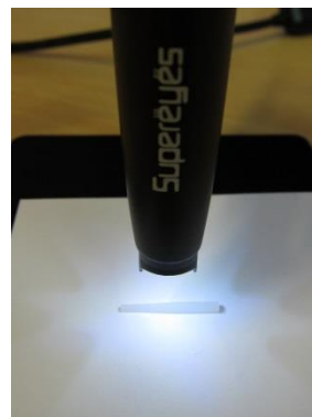
Fig 4. Digital microscope and digital caliper used in the study.
