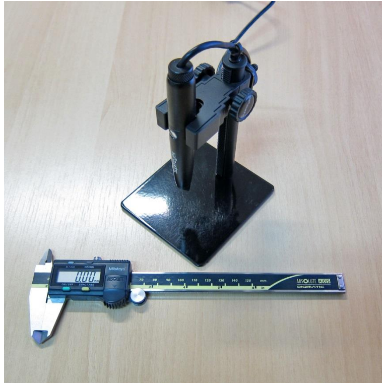
Fig 4. Digital microscope and digital caliper used in the study.
