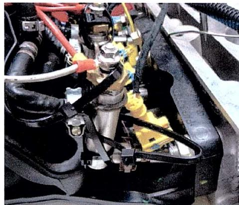
Figure 3 - Detail of fuel distributor with electrical injectors.
