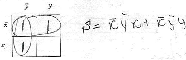
$S = \bar{x} \bar{y} \bar{y} + \bar{x} \bar{y} y$
